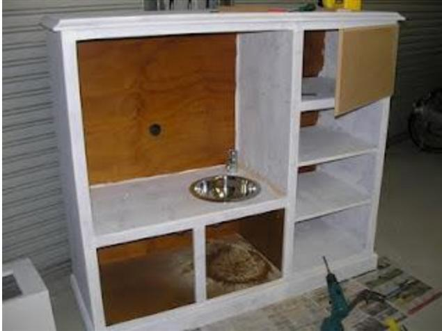
A hole was cut in the shelf where the TV once sat and a tap was added. The fridge and freezer were fitted for their doors. Then another coat of paint.
